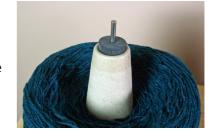
Inspect your work and make sure no portion of the cone is making contact with the wooden YPT base. Also make sure the cone turns freely by spinning it. If not, check your collars on the wooden disc.
