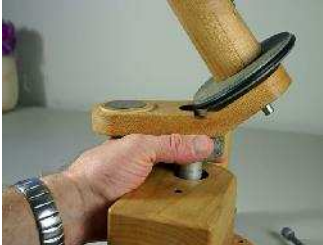
Do not touch the spindle at this point. Only support the Arm.
