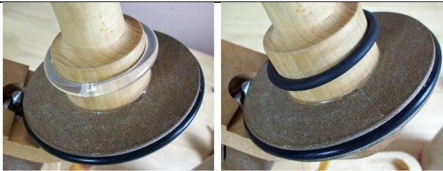
The O-rings are simply inserted onto the thicker portion of the spindle, about halfway up from the bottom. They will stay in place when you are inserting and removing cones. If they shift in position, simply adjust them. The clear o-ring is used with our cones.
